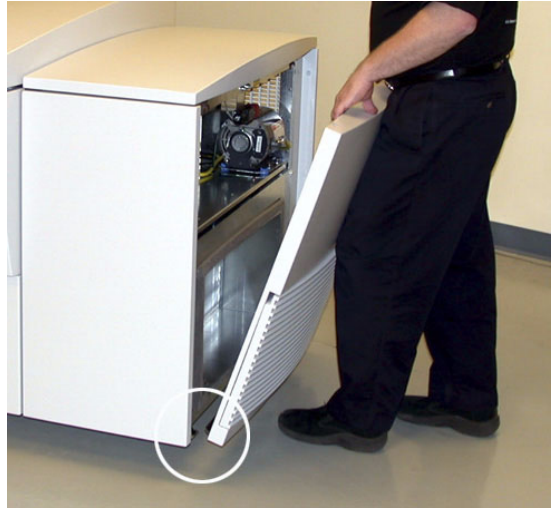
Figure 14: Replace the fan box panel
