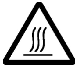
Figure 49: Hot Surface Caution label
