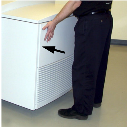
Figure 13: Remove the fan box panel
